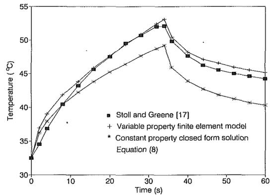
Fig. 1 Basal layer temperature-time histories determined using finite element and closed-form solutions and reported by Stoll and Greene [17] (exposure of 4.186 kW/m<sup>2</sup> for 34 s)
