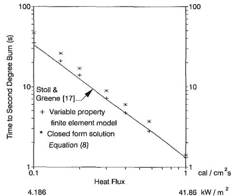
Fig. 2 Times to second degree burn as predicted by finite element and closed-form solutions, and observed by Stoll and Greene [17]
